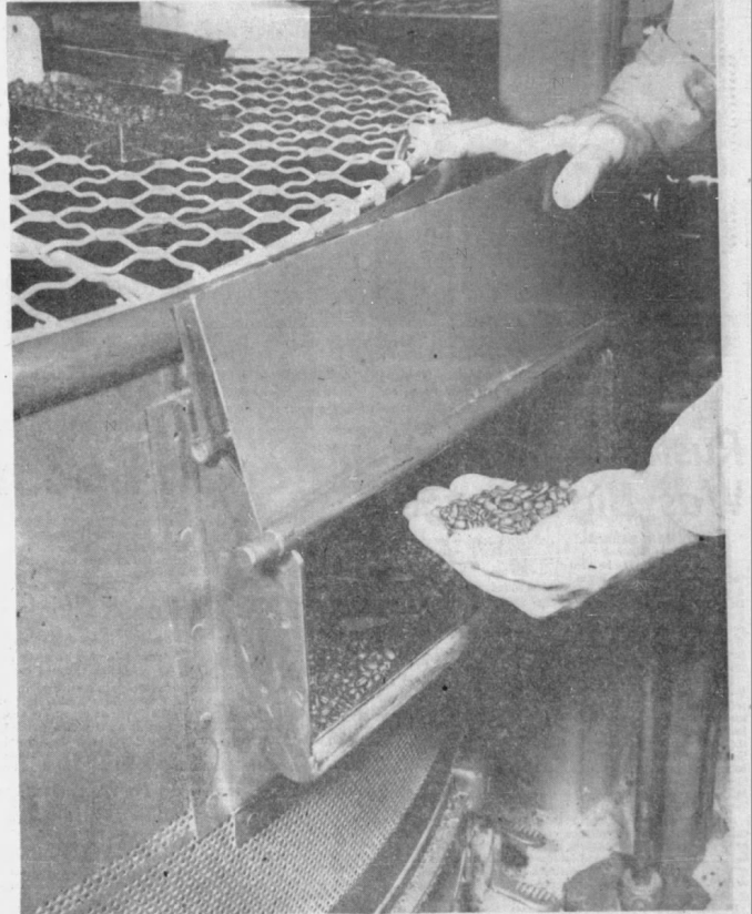
HUMAN HANDS CHECK the performance of machinery. This test is to determine whether the coffee is sufficiently cool for the next step in the processing.
