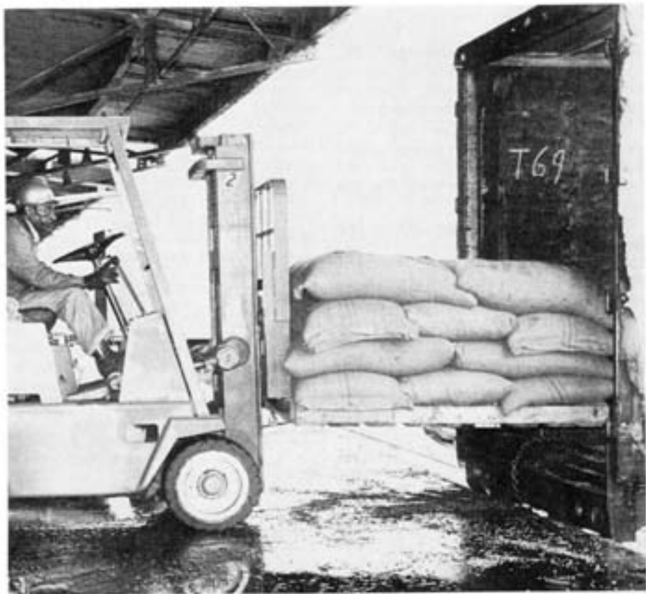
Palletized coffee bags are lifted into truck to be taken to roasting plants
